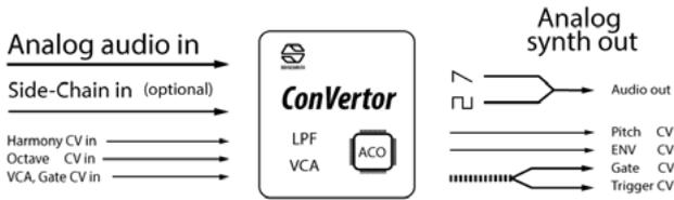
In the ConVector all the audio inputs are accommodated via mono instrument jacks (TS) at the back panel and all the CV inputs and outputs are accommodated via mono mini jacks on the front panel. The only stereo mini jack is the gate/trigger output which shares a stereo mini jack. Plug a mono mini jack to have the gate output, or use a stereo Y cable to split the Gate CV from the L channel and the trigger CV output from the R channel.
